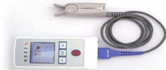
Figure 10. Medical Information Tag, or miTag- is a Tmote mini-based patient monitor that includes a pulse oximetry sensor with LEDs, buttons and an LCD screen. The miTag is powered using a rechargeable 1200-mAh, 3.7-V Li-Ion battery and external finger tip sensors are used to make the pulse oximetry measurements,
